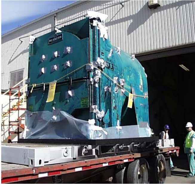
CC Fix Stabilized this Uranium and Beryllium Contaminated Furnace
